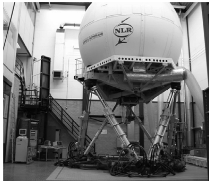
Fig. 2 NLR research flight simulator (GFORCE) with the six-DOF motion system in its neutral position (left), and prepositioned for simulation of direct motion (right).
