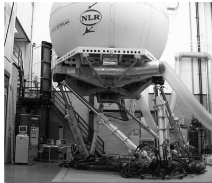
Fig. 2 NLR research flight simulator (GFORCE) with the six-DOF motion system in its neutral position (left), and prepositioned for simulation of direct motion (right).
